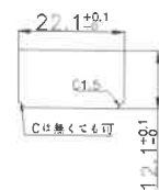
取付穴参考図 Size of mounting hole
