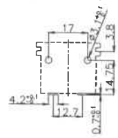
取付穴参考図 Size of mounting hole
